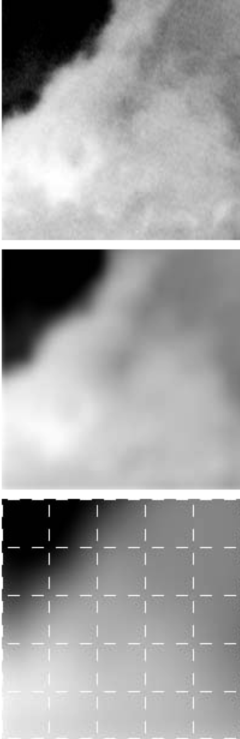
Fig. 2 Zoomed-in refractive-index-field region, extracted from a whole image, showing resolution reduction by coarse-graining using biquadratic B-splines; reference resolutions of (top) 200 by 200 pixels, (middle) 20 by 20 pixels, and (bottom) 5 by 5 pixels.
